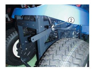
2. If you dismount the grass collector from machine before installing mower deck SMM54, remove harness (for safety switch) (3) from connector (2).
