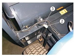
3. Connect the Connector / Joint ASSY (1) to connector (2).
